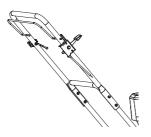
**Dead-man's handle:** This handle is mounted on the handlebar and must be pressed in order to start the engine. Releasing the handle disengages the engine.
