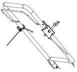
• The air velocity can be controlled by adjusting the engine regime. This is done by decreasing throttle.
