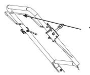
In case of an emergency, simply release the dead-man's handle: this will cut off the engine.
